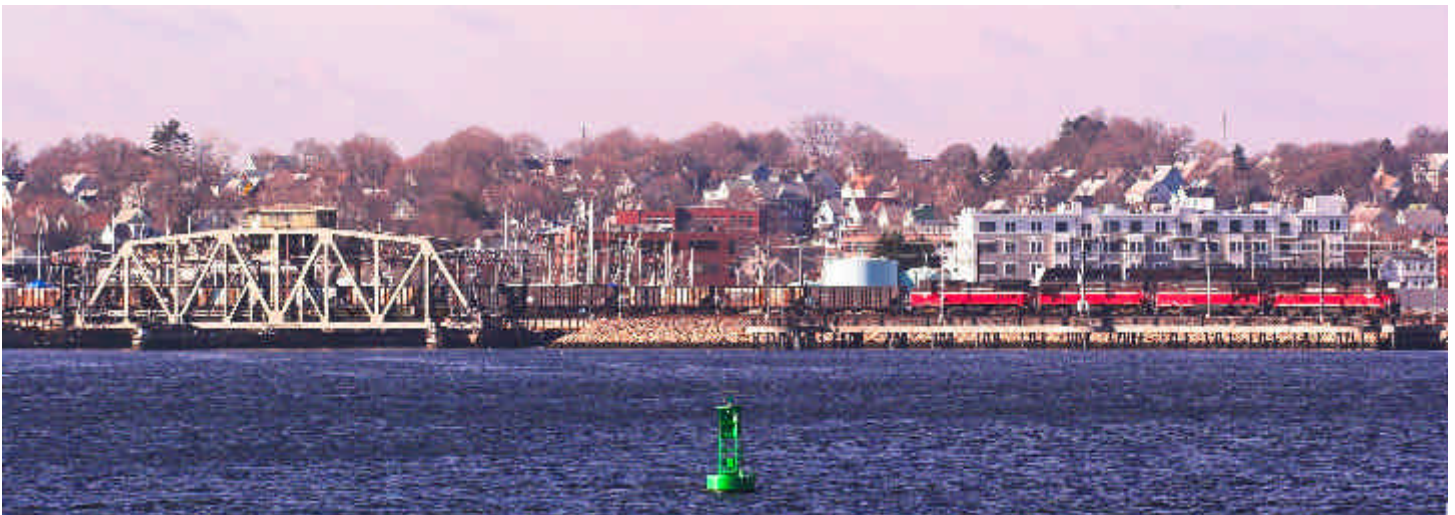
New London, Connecticut. PW coal train #3 to Johnson City 25 January, moving east at Shaw's Cove, heading for the NECR yard. The train must back up this far to trigger the signal permitting it to run off the Amtrak line just east of the depot. Photo by Thomas J. Nanos www.nanosphoto.com
