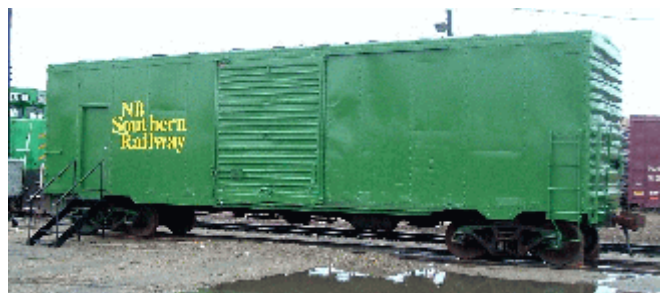
McAdam, New Brunswick. NBSR's newly-painted boxcar serving as transload dock. Trucks back to car door show, pulp passes through to railcar via door on opposite side. {courtesy Steve Boyko 11.Mar.06}
