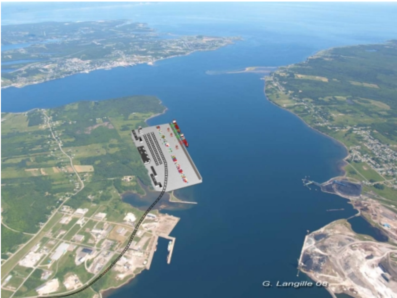
Sydney harbor, proposed container terminal. The land area would be created by dredging a channel in the outer harbor (at the top of the picture). About half the rail spur already exists. {Sydney Marine Group, Chicago presentation}
